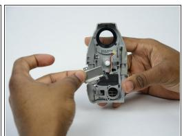
Remove the metal plate. This metal plate protects the black speaker holder.
