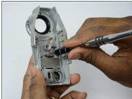
Take the front panel and remove the three 2.75 mm screws from the metal plate.
