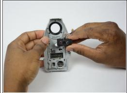
Remove the black speaker holder from the front panel. This holds the individual speakers.
