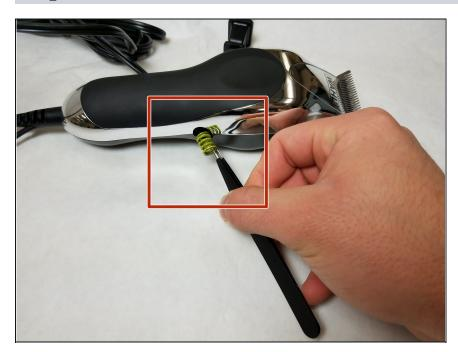
Remove the spring on the side of the body using tweezers.
