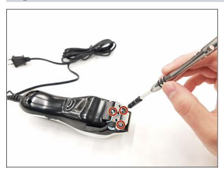
Remove the three 9.0 mm JIS #1 screws attaching the base of the blade assembly to the body.
