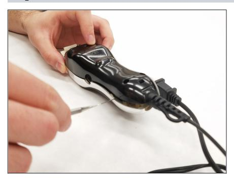
Pry the body case off of the device using a spudger.
