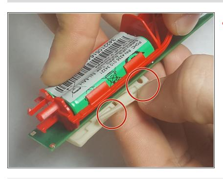
Remove the white circuit board cover as shown. This cover will require you to pry off the piece from the groves.
