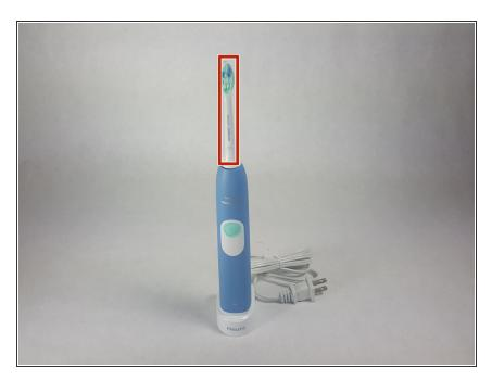
Pull upwards to remove the brush head from the top of the device.
