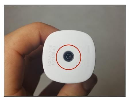
Remove the 12 mm T8 Torx screw from the bottom of the toothbrush.
