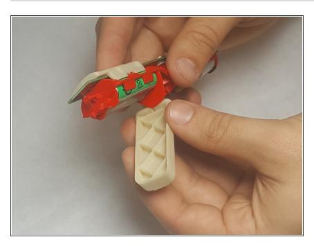
Remove the white battery cover as shown in the figure.
