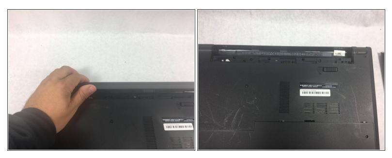
• Rotate the battery up and remove it.
