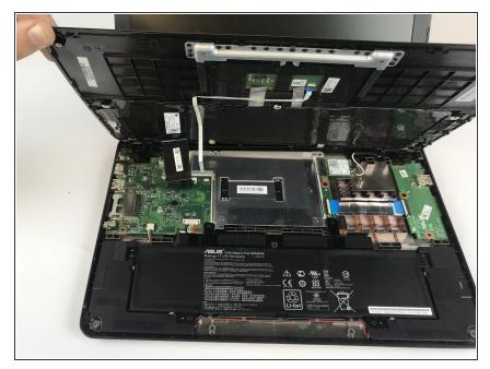
Use plastic opening tool to pry open clip holding keyboard wires to the circuitboard.
