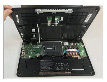
Lift and remove keyboard from device.
