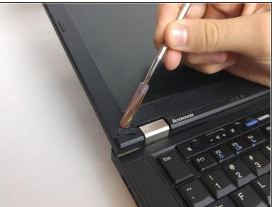
Use a spudger to remove the plastic covers from the LCD screen.
