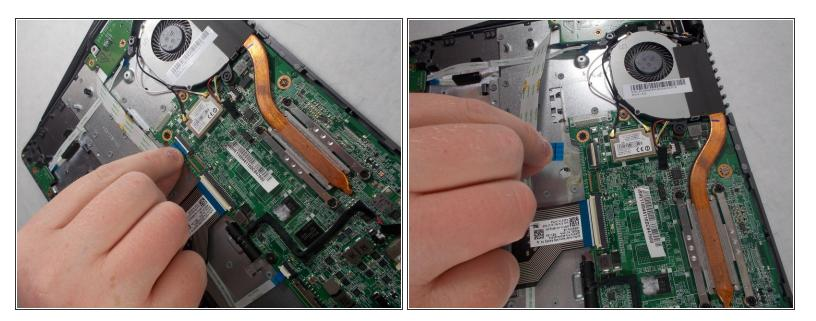
• Pull the blue tab on the ribbon cable to remove it.
