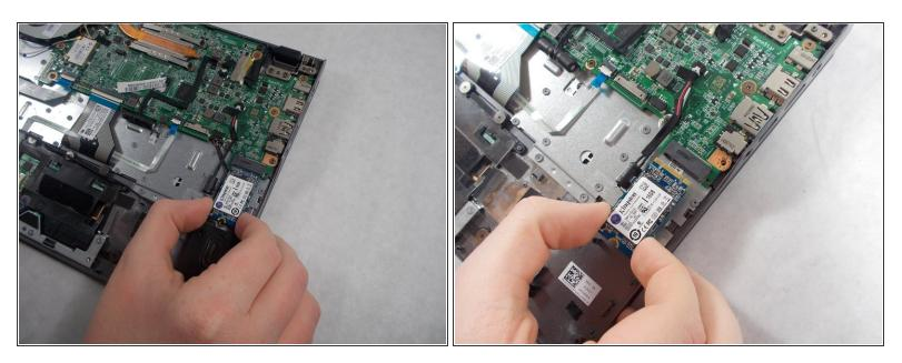
• Carefully pull out the solid state drive using two fingers.
