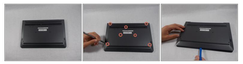
A Make sure that device is fully powered down before attempting to open the back case.
