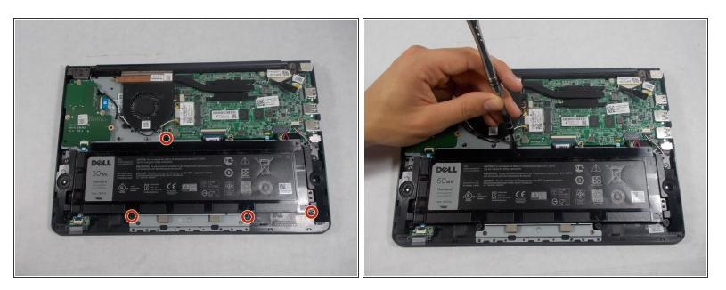
• Use a Phillips #0 screwdriver to unscrew the four 8 mm screws that secure the battery.
