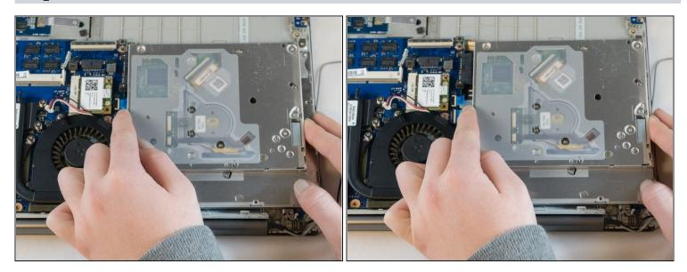
• Place your fingers on either side of the optical drive and slide it away from the fan to remove it.
