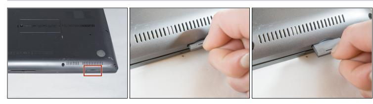
Using your fingers, pinch the edge of the SD card and pull to remove it.
