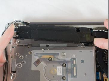
• With your fingers, grasp the edges of the speaker and slide it up and away from the fan to lift it out of the case.
