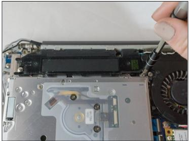
Using the Phillips#00 remove the three 3.5mm screws that secure the speaker to the bottom case.
