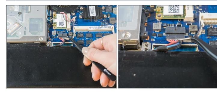
• Using <u>tweezers</u> or your fingertips, carefully pull on the battery connector to disconnect it from the motherboard.
