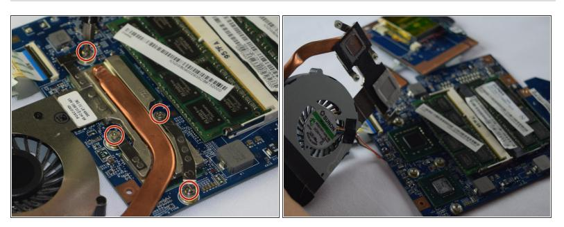
Remove the four (4) screws that are holding the CPU's cover on
