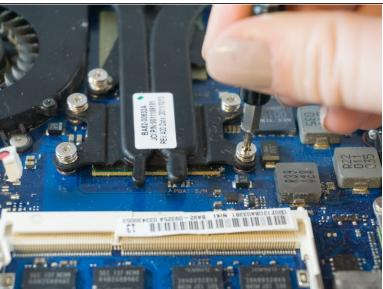
• Loosen but don't remove the 7 silver Phillips #00 3.5mm screws securing the fan to the motherboard. They should detach from the motherboard and remain attached to the fan assembly.
