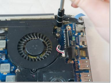
• Using the Phillips#00 remove the four 3.5mm screws securing the fan to the motherboard.
