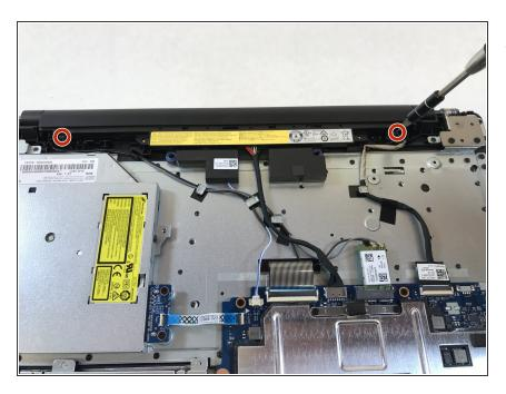
Remove the two 9 mm Phillips #1 screws holding the battery.
