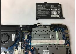
Carefully disconnect the cable connecting the top of the battery and remove the battery.
