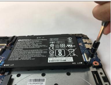
Using a PH0 screwdriver, unscrew the two 3.8mm PH0 Phillips head screws that hold the battery in place.
