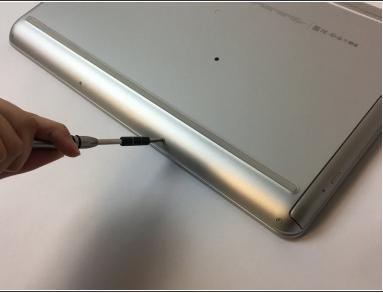
Using a PH0 screwdriver, unscrew the ten 4.4mm Phillips head screws located on the back panel.
