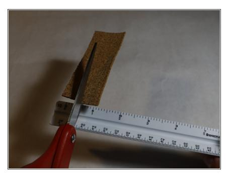
• Cut the new cork to match the width of the tenon joint.
