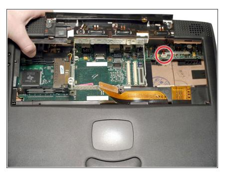
Grasp the upper case near the back left corner and lift up partly so that you can access and disconnect the
